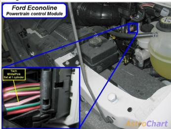
The PCM is under the hood, next to the brake master cylinder.
